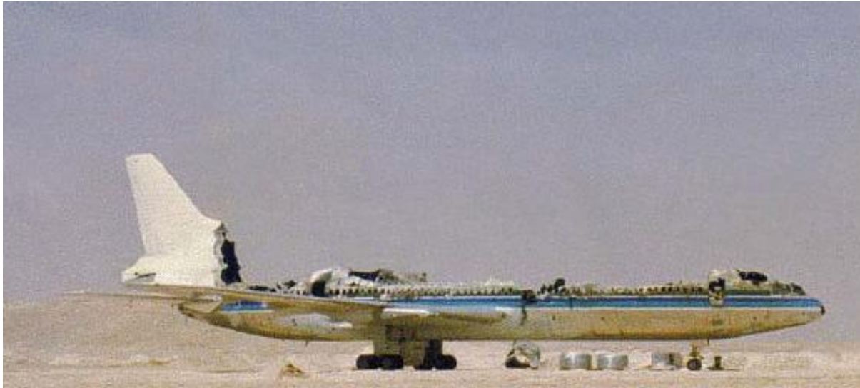
Fig 1: The burnt-out hulk of Saudi Airlines Flight 163 remained at Riyadh airport for several years. The engines were removed after the accident. (Michael Busby)
