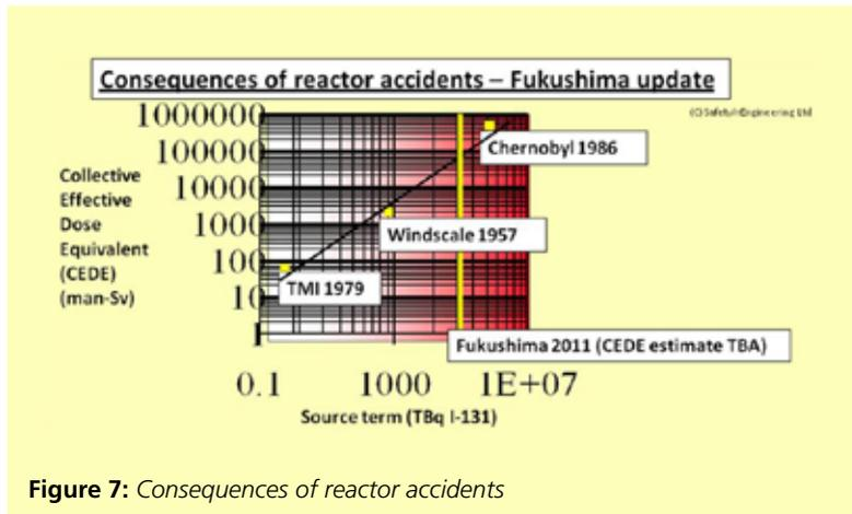
Figure 7: Consequences of reactor accidents
