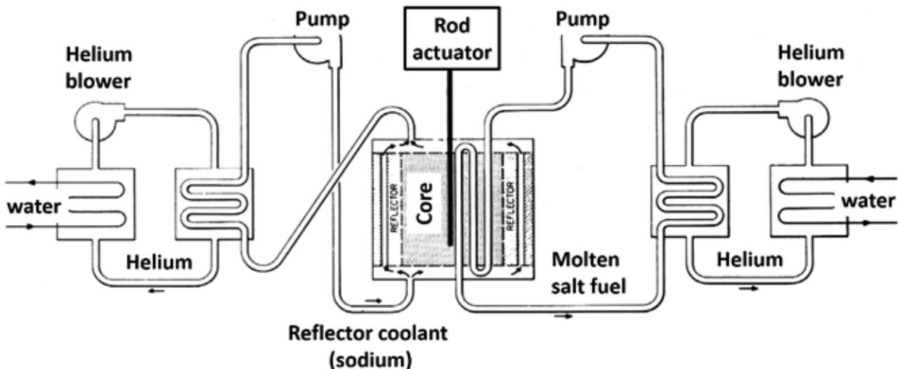
**FIGURE 1: A schematic diagram of the land-based Aircraft Reactor Experiment (ARE), which was operated during November 1954 at Idaho National Laboratory [2]. Separate loops for reactor cooling (molten salt to helium) and BeO reflector cooling (sodium to helium) are shown.**
