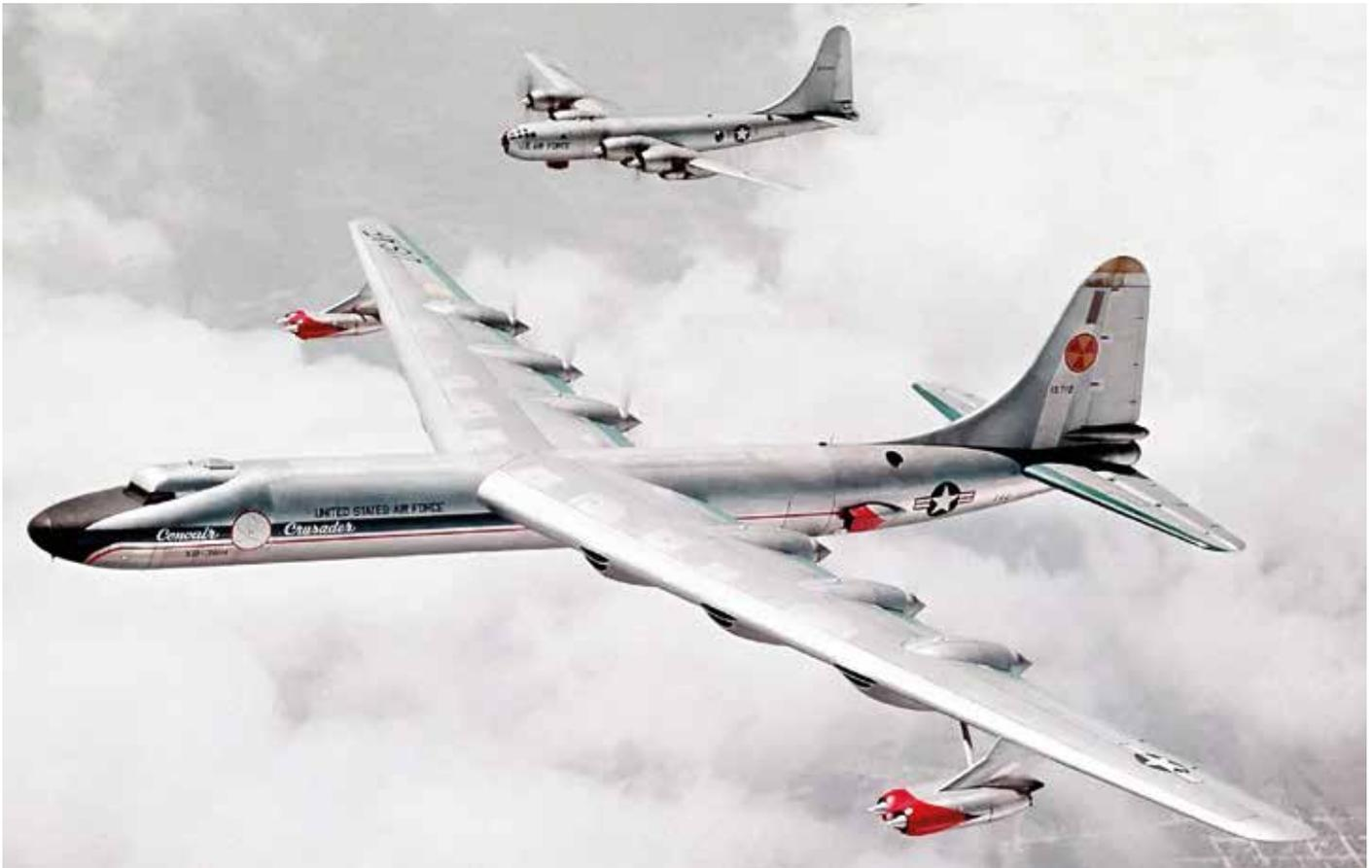
**FIGURE 2: The Convair NB-36H Crusader with the Aircraft Shield Test Reactor – the only US aircraft to have flown while carrying an operational nuclear reactor. The radiation symbol can be seen on the vertical stabiliser. A Boeing B-50 Superfortress chase aircraft is also shown, which indicates the size of the NB-36H. (USAF)**
