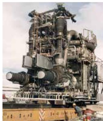
**FIGURE 5: HTRE-3 powered the first true nuclear-powered turbojets. It was a ground-based prototype for possible use in an aircraft. It produced significant jet thrust and was able to start itself using nuclear heat. It suffered a fuel melt in its first few weeks of operation in November 1958; the core was replaced, and it was operated until early 1961. (Idaho National Laboratory)**
