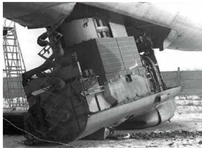
**FIGURE 10: The Tupolev Tu-95LAL reactor shielding test carried the 100kW VVRL-100 reactor in its bomb bay during 34 flights in 1961.**
