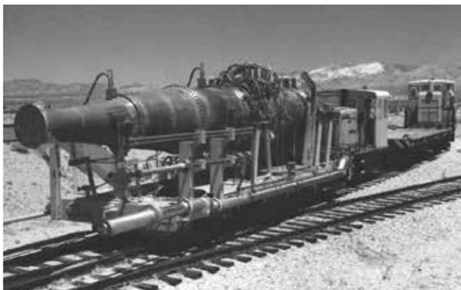
**FIGURE 8: The Tory-IIC nuclear ramjet which was successfully tested in Idaho in May 1964.**
