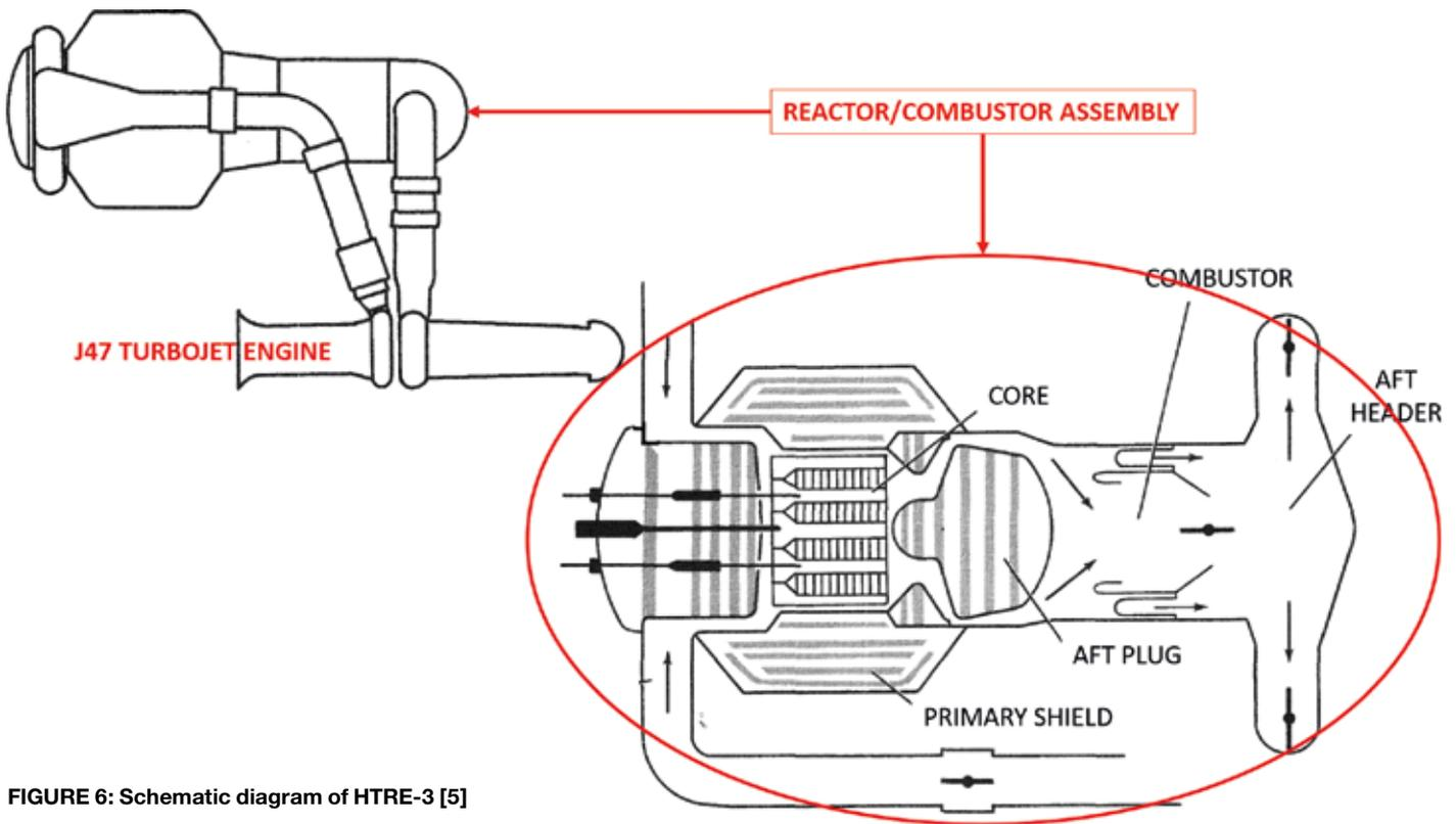
FIGURE 6: Schematic diagram of HTRE-3 [5]
