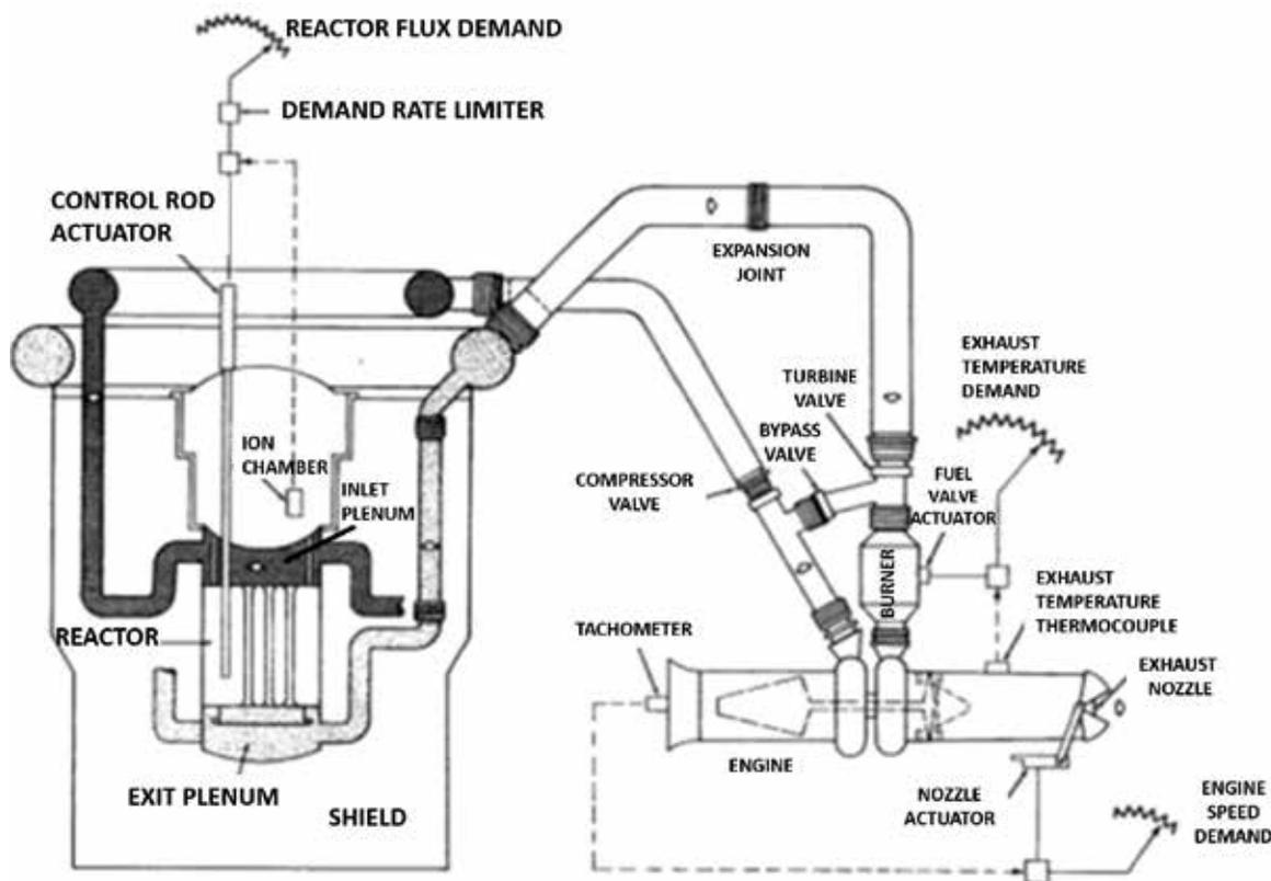
FIGURE 3: Schematic diagram of HTRE-1/HTRE-2. The turbojet was started up using jet fuel and only then switched over to nuclear heat [4]
