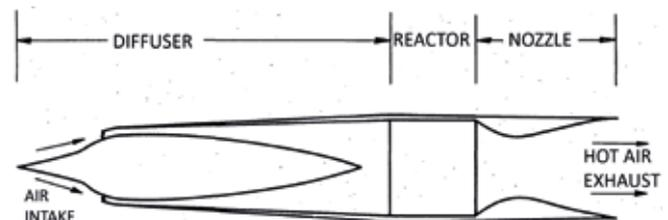
FIGURE 7: Conceptual layout of a nuclear-powered ramjet.
