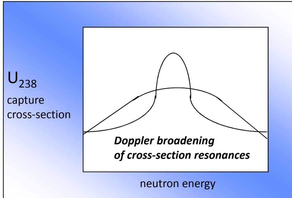
**Doppler Broadening** – as U-238 gets hotter, the resonance peaks broaden due to vibration of the nuclei. The net effect is that U-238 absorbs more neutrons (*without causing fission*) as the reactor temperature increases. Hence an increase in reactor temperature leads to a fall in reactivity.
