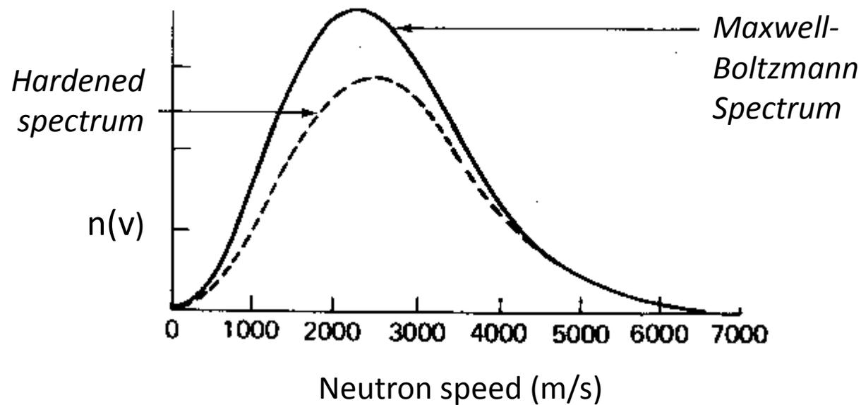
The Maxwell-Boltzmann distribution for thermal neutrons
