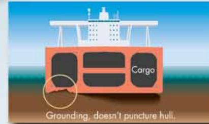
Grounding, doesn't puncture hull.
