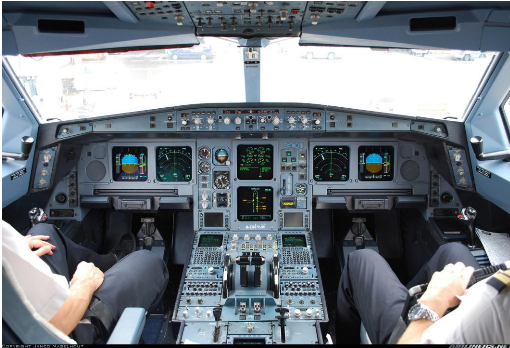
11-4: Airbus A330 cockpit showing the positions of the control sticks for the two pilots, on the extreme right and extreme left. ( www.airliners.net )
