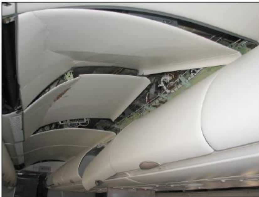
Fig 3: This photo shows some of the damage to the cabin roof caused by passengers being thrown upwards by the sudden pitch down of Qantas flight 72.
