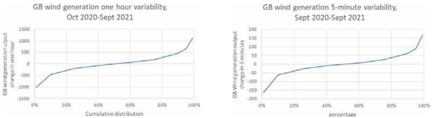
FIGURE 8: Variability of GB wind turbine fleet output at one-hour (left) and 5-minute (right) intervals, October 2020 to September 2021. The diagrams present the probabilities of variations of wind turbine fleet output within the defined timescales. (Author’s analysis based on data from Gridwatch.)
